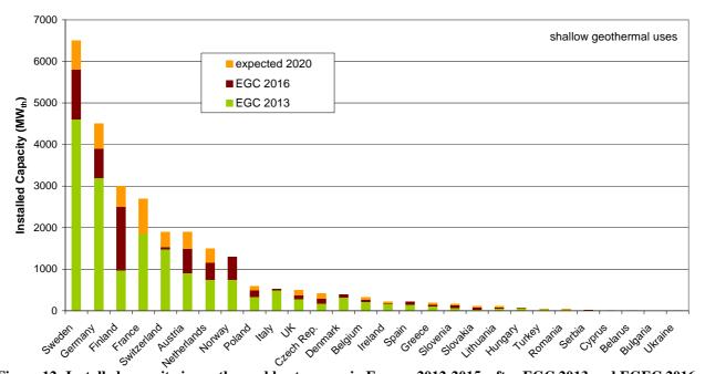
Figure 12: Installed capacity in geothermal heat pumps in Europe 2012-2015, after EGC 2013 and EGEC 2016, and reported expectations towards 2020 (EGC-2016-values for Denmark from WGC 2015)
