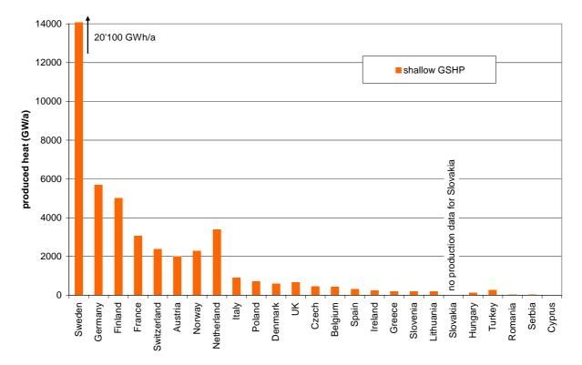
Figure 19: Visualisation of data on installed capacity and produced heat from table 4 (values for Denmark from WGC 2015)
