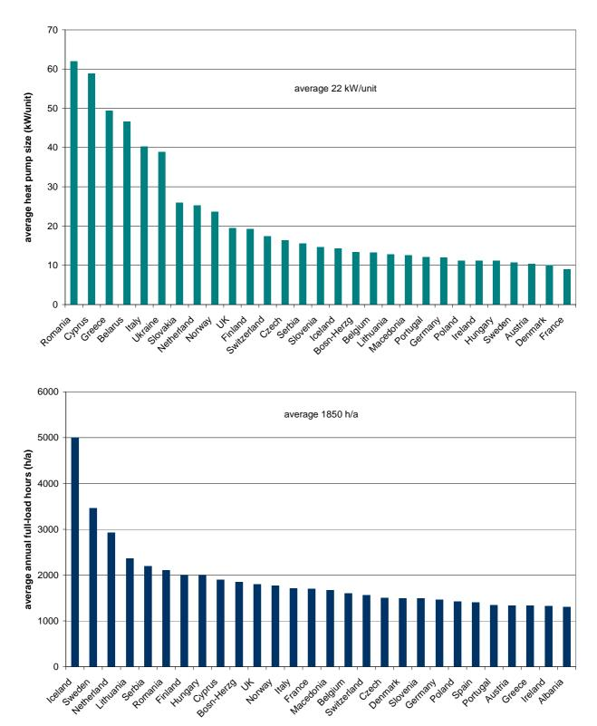
Figure 20: Average heat pump size (top) and annual full-load hours (bottom) for ground source heat pumps
