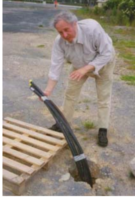
Figure 3: Test BHE at the site Wetzlar-Spilburg, ready for Thermal Response Test (photo Lund, June 2004)
