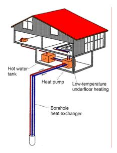
Fig. 3: Typical application of a BHE / heat pump system in a Central European home, typical BHE length ≥100 m
