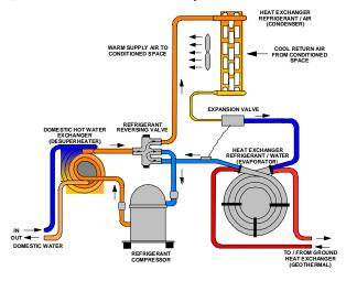
Figure 1b. Water-to-air GHP in the heating cycle (source: Oklahoma State University)
