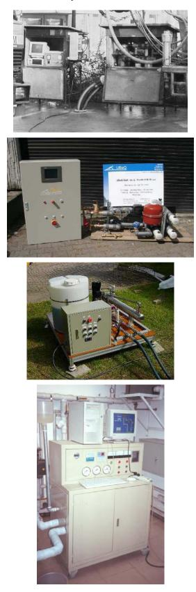
Fig. 7: Different thermal response test rigs, from above: Early rig from Landtechnik Weihenstephan, rig built by UBeG for export to China, light rig built by hp system tech in South Korea, laboratory rig at Beijing University of Technology, China
